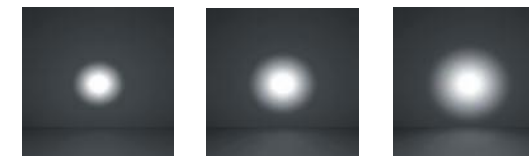
S - Spot α 14° M - Medium α 28° WF - wide Flood α 40°
